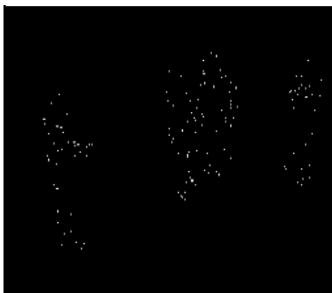
Below: Image from above after threshold filtering shows only the markers.
